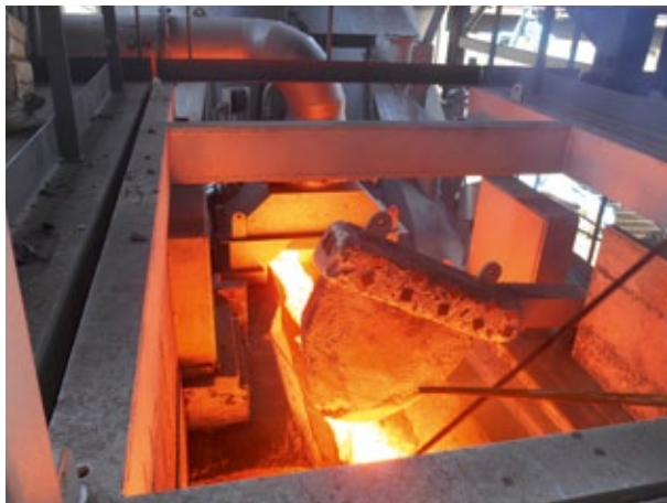
Slag flowing to granulator, photo: Primetals Technologies
