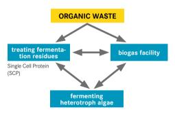
algae, all in a single facility. Fermentation residues from producing biogas are used to make customized fertilizers and high-grade protein feed. Two-thirds of the remaining fermentation residues are converted into clean water, and
