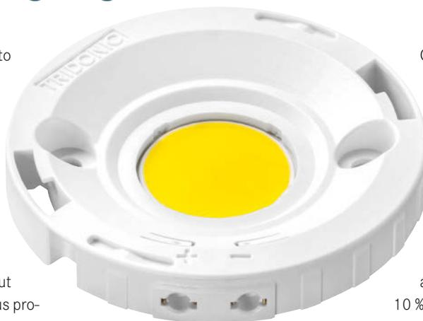
On the basis of these research activities Tridonic Jennersdorf GmbH launched the LED module TALEXX engine STARK SLE as a sustainable system solution for LED downlights and spotlights; this product is remarkably efficient (156 lumen/watt) and achieves a service life of 50,000 hours with a decline in luminous flux of at most 10 %. Over 960,000 LED-modules have been produced so far with substrates developed in the ADLED-project.
