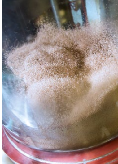
Close-up of fluidized-bed stage in adsorber, Photo: TU Wien/Julius Pirklbauer
