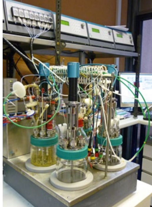
Top left: wood sample after steam explosion to break up its structure. Top centre: enzymatic hydrolysis of wood to release the sugars. Bottom left: the yeast Candida lignohabitans , which converts these sugars into exploitable substances. On right: a laboratory fermentation unit in which the yeast performs this conversion. Photos: University of Natural Resources and Life Sciences, Vienna, Department of Biotechnology
